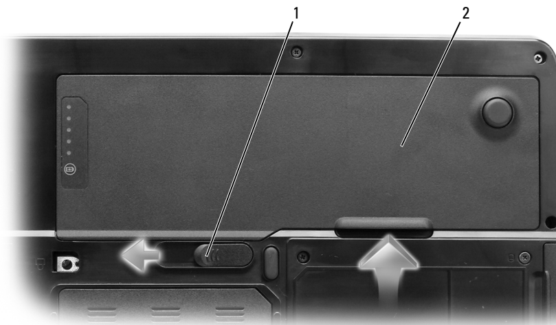
1 battery-bay latch release 2 battery
